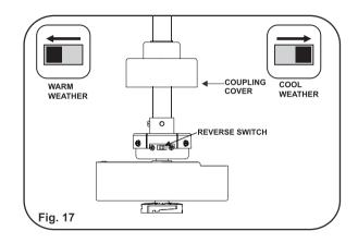
Warm Weather(forward) A DOWNWARD airflow creates a cooling effect as shown in Figure 16. This allows you to set your air conditioner on a warmer setting without affecting your comfort.
